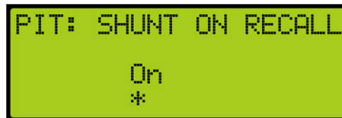
Figure 593: PIT: SHUNT ON RECALL Menu
