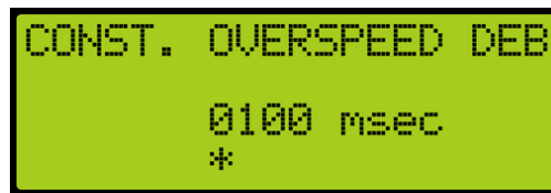
Figure 516: CONSTRUCTION. OVERSPEED DEBOUNCE Menu
