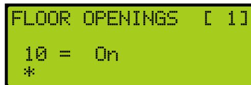
Figure 276: FLOORS OPENINGS (Rear) Menu
