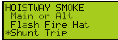
Figure 575: HOISTWAY SMOKE Menu – Shunt Trip
