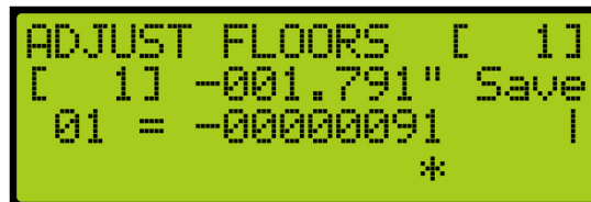
Figure 228: ADJUST FLOORS Menu – Too High
