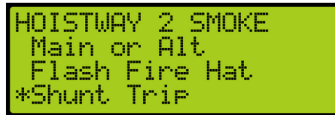
Figure 601: HOISTWAY 2 SMOKE Menu – Shunt Trip
