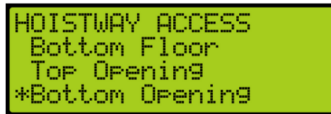
Figure 407: HOISTWAY ACCESS – Bottom Opening
