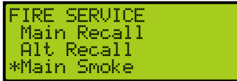
Figure 556: FIRE SERVICE Menu – Main Smoke
