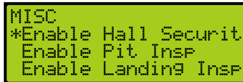
Figure 371: MISCELLANEOUS Menu – Enable Hall Security
