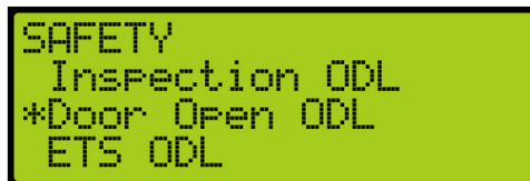
Figure 509: SAFETY Menu – Door Open ODL
