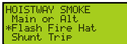
Figure 573: HOISTWAY SMOKE Menu – Flash Fire Hat
