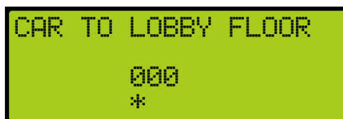
Figure 429: CAR TO LOBBY FLOOR Menu
