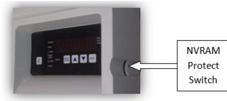
Figure 9: NVRAM Protection Switch
