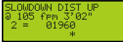
If adjusting the car for a different threshold with weights added and the car is overshooting or the leveling time is greater than the empty car, increase or decrease the slowdown distance.
