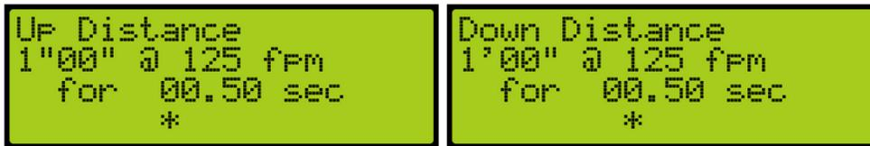
3. Scroll back to GENERATE THRESHOLDS AND DISTANCES and select YES. If YES is not selected, new thresholds and slowdowns are not generated.
