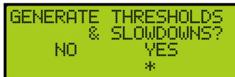
4. Selecting yes will generate the values for slowdown distance up, slow down distance down, and threshold.
