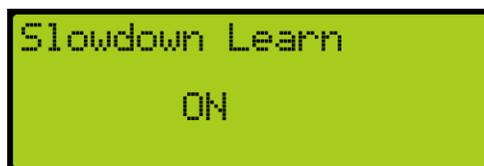
4. Allow the car to run from Floor to Floor for 2 full cycles to adjust the slowdown distance. It is recommended to run the car empty during the first 2 cycles to allow the car to measure the slowdown distance accurately.
