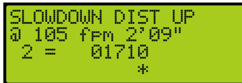
3. The high speed of the car must be less than the speed threshold. For example, after adding weights the high speed of the car is 100 fpm, select the speed threshold with speed of 105 fpm.
