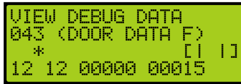
Figure 240: VIEW DEBUG DATA Menu – Front Door
