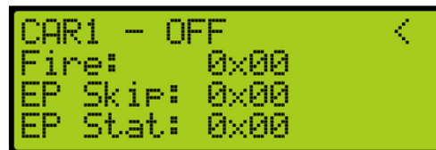
Figure 589: Fire Emergency Power Status Menu
