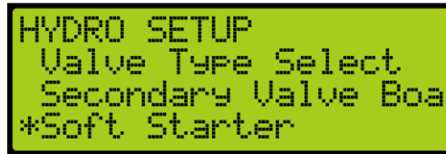
Figure 282: HYDRO SETUP Menu –Soft Starter
