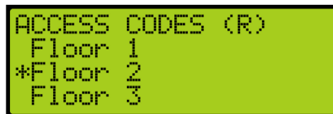
Figure 129: ACCESS CODE REAR Menu – Floor Number
