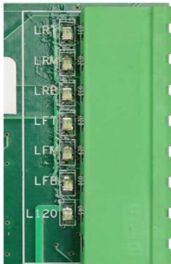
Figure 21: Hall Lock Connector
