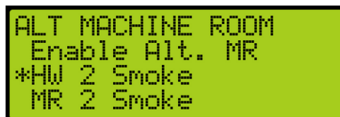
Figure 501: ALT MACHINE ROOM Menu – HW 2 Smoke
