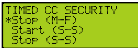
Figure 152: TIMED CAR CALL SECURITY Menu – Stop (M-F)
