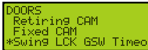
Figure 234: DOORS Menu – Swing Lock GSW Timeout
