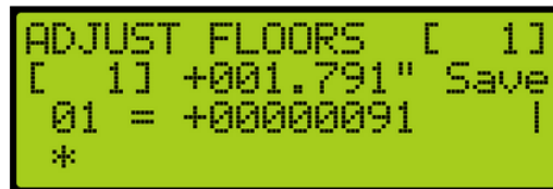
Figure 123: ADJUST FLOORS Menu – Too Low
