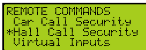
Figure 560: REMOTE COMMANDS Menu – Hall Call Security
