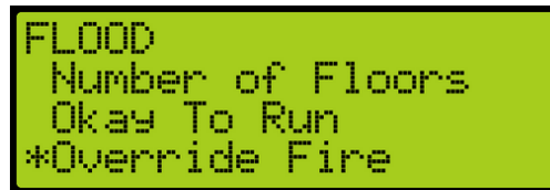
Figure 515: FLOOD Menu – Override Fire
