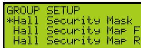
Figure 268: GROUP SETUP Menu – Hall Security Mask
