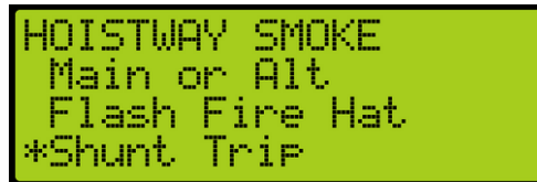
Figure 487: HOISTWAY SMOKE Menu – Shunt Trip
