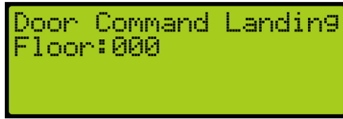
Figure 569: Door Command Landing Menu
