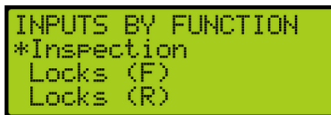
Figure 527: INPUTS BY FUNCTION Menu –Inspection
