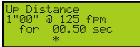
Figure 328: Up Distance Menu – Steady State of Leveling Longer Adjustment
