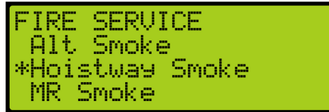
Figure 484: FIRE SERVICE Menu – Hoistway Smoke
