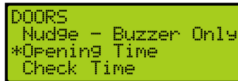
Figure 222: DOORS Menu – Opening Time
