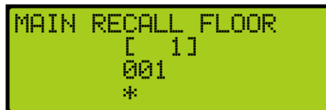
Figure 464: MAIN RECALL FLOOR Menu
