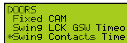
Figure 236: DOORS Menu – Swing Contacts Timeout
