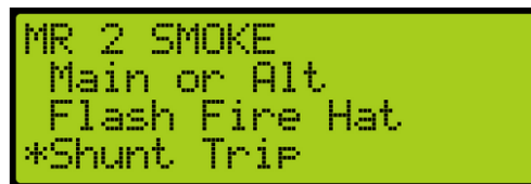
Figure 508: MR 2 SMOKE Menu – Shunt Trip
