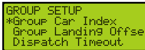
Figure 573: GROUP SETUP Menu – Group Car Index
