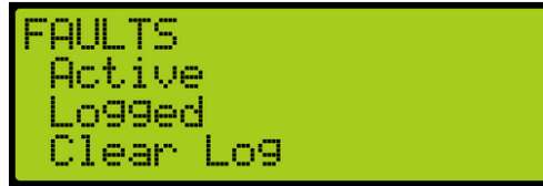
Figure 52: FAULTS Menu – Active, Logged, Clear Log
