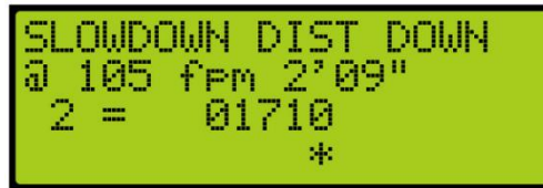
Figure 339: SLOWDOWN DISTANCE DOWN – Adjustment
