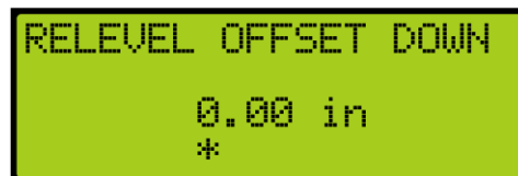
Figure 314: Relevel Offset Down Menu
