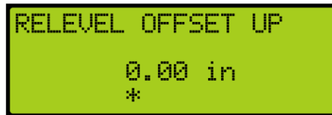
Figure 313: RELEVEL OFFSET UP Menu
