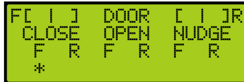
Figure 182: CONTROL DOORS Menu
