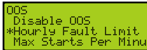
Figure 397: OOS Menu – Hourly Fault Limit
