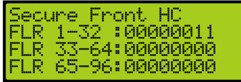
Figure 562: Secure Front Hall Call Menu
