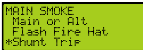
Figure 477: MAIN SMOKE Menu – Shunt Trip
