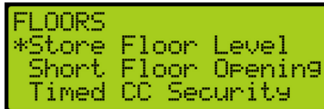
Figure 144: FLOORS Menu – Store Floor Level
