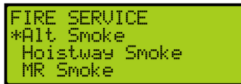
Figure 479: FIRE SERVICE Menu – Alt Smoke
