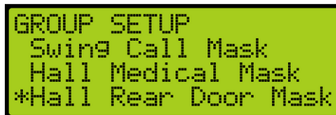
Figure 274: GROUP SETUP Menu – Hall Rear Door Mask
