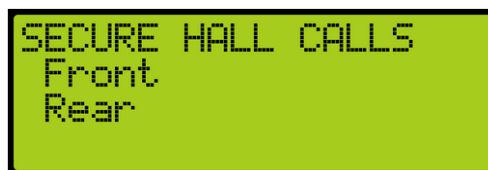
Figure 561: SECURE HALL CALLS Menu – Front or Rear
