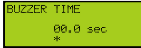
Figure 594: BUZZER TIME Menu
