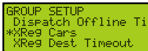
Figure 581: GROUP SETUP Menu – XREG Cars
