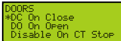
Figure 202: DOORS Menu – DC On Close
