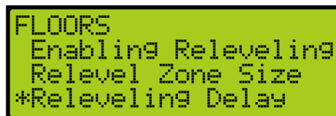
Figure 140: FLOORS Menu – Releveling Delay
