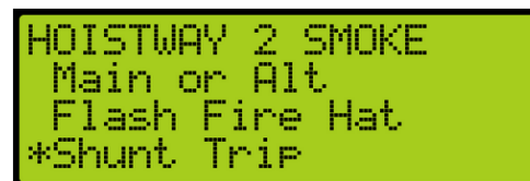
Figure 504: HOISTWAY 2 SMOKE Menu – Shunt Trip
