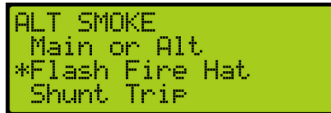
Figure 482: ALT SMOKE Menu – Flash Fire Hat
