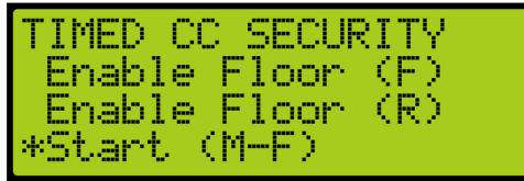
Figure 150: TIMED CAR CALL SECURITY Menu – Start (M-F)
