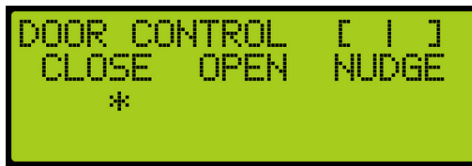
Figure 602: Enter Door Command Menu (Front Doors Only)
