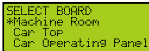
Figure 159: SELECT BOARD Menu – Machine Room
