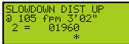
Figure 338: SLOWDOWN DISTANCE UP – Adjustment
