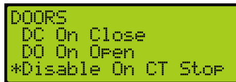
Figure 206: DOORS Menu – Disable On CT Stop
