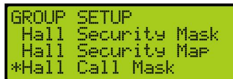
Figure 270: GROUP SETUP Menu – Hall Call Mask
