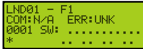
Figure 276: Hall Lantern Status
