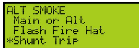
Figure 483: ALT SMOKE Menu – Shunt Trip
