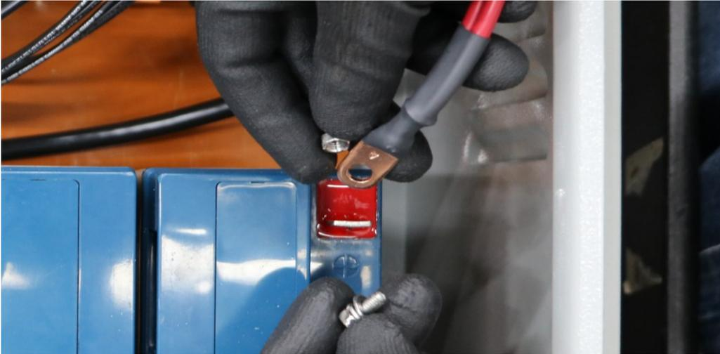
*Figure 9: Remove Power and Ground Cable*
