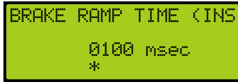
Figure 57: BRAKE RAMP TIME (INSP) Menu
