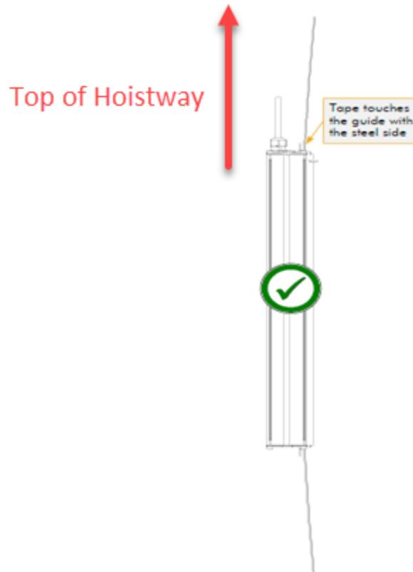
Figure 4: Magnetic Tape Installation<sup>1</sup>
