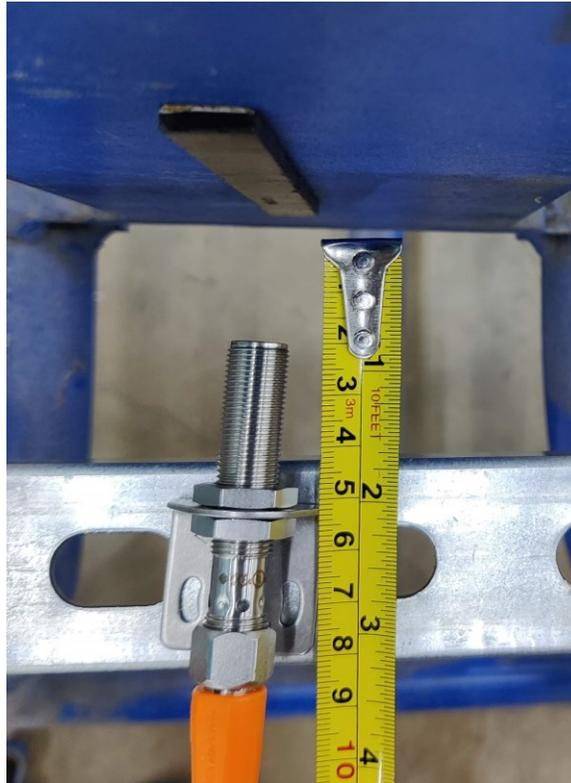
Figure 2: Mounting Proximity Sensor Assembly (Example)
